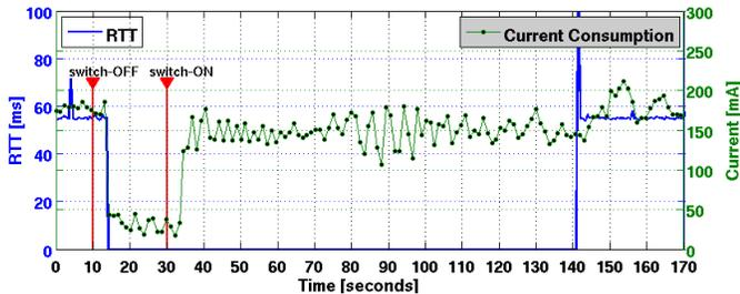
Figure 3: Switching time: measurements for a sample WAD.
