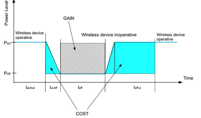
Figure 2: Graphical representation of the energy saved and of that wasted due to switching time. During switching, the device spends additional energy  $E_{act-off} + E_{off-act}$ , which we refer to as cost.
