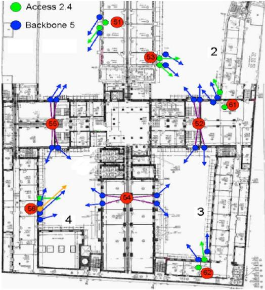
Figure 5: Network topology for testing scenarios. The red dots represent the WiFi APs used in our experiments. The green and blue dots and arrows show the antenna directions for access and backbone interfaces, respectively.
