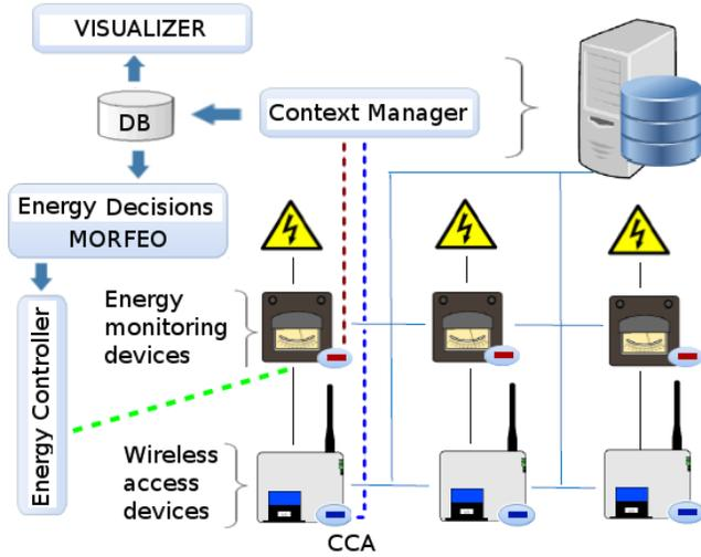
Figure 1: Our energy monitoring and control framework. MORFEO is an example of energy-decision algorithms used to drive energy-saving actions in a wireless infrastructure network.
