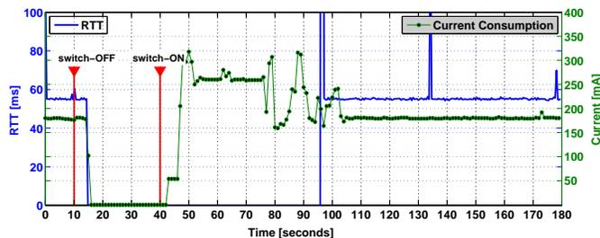
Figure 4: Switching time: measurements for a sample WAD<sub>2</sub>.
