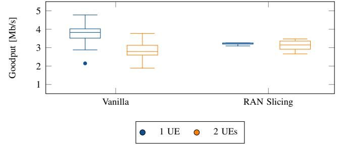
Fig. 12. Performance comparison for 2 UEs with the same signal quality and 2 network slices with 50% of the resources.
