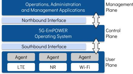
Fig. 1. The high-level view of the *5G-EmPOWER* architecture.
