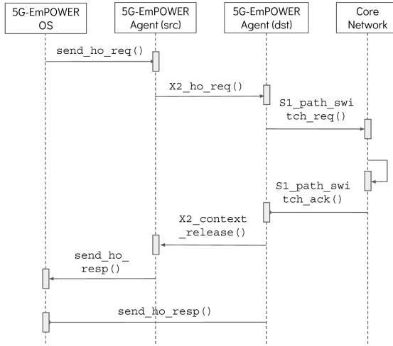
Fig. 17. Procedure handled by *5G-EmPOWER* to perform an X2 handover.
