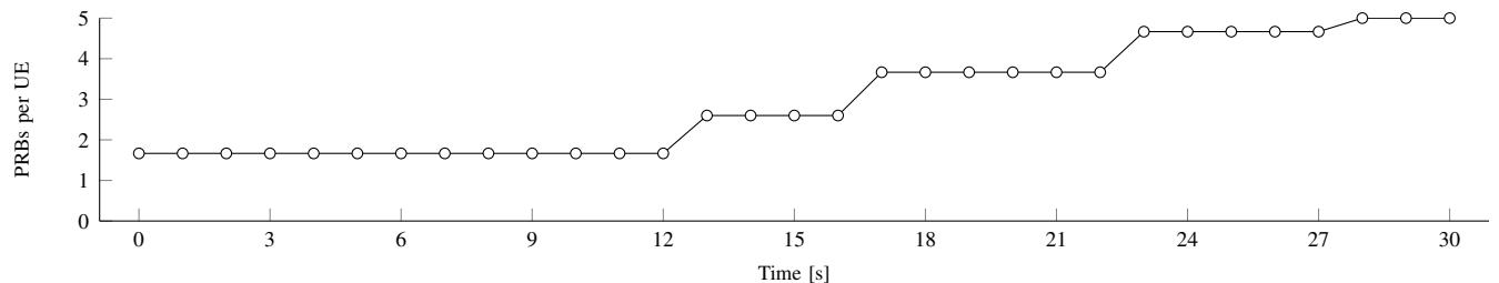
Fig. 20. Average number of PRBs per UE assigned in 4 eNBs for during 30s while 15 UEs are distributed across the network to balance the traffic load.
