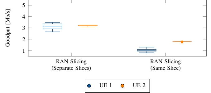
Fig. 15. Performance evaluation of the RAN slicing solution with 2 UEs and 2 network slices. In the first test the UEs are located in separate slices, while in the second one they share the same slice.
