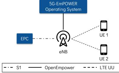
Fig. 8. Network topology used for the performance and overhead evaluation.
