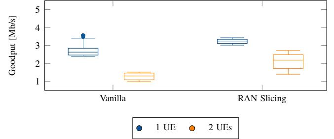
Fig. 13. Performance comparison for 2 UEs with different signal quality with 2 network slices with 50% of the resources.
