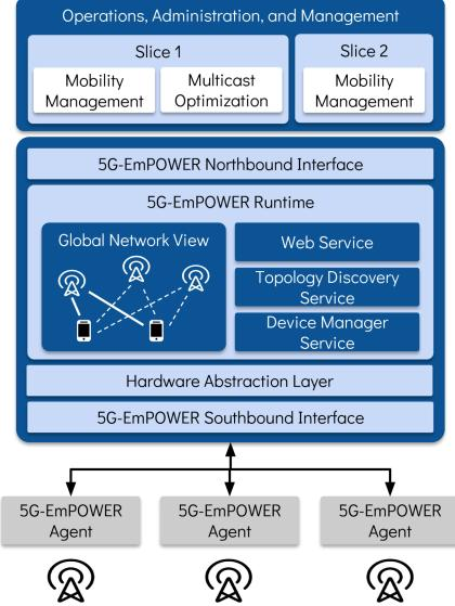
Fig. 5. The 5G-EmPOWER Operating System.
