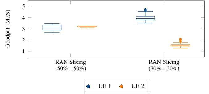
Fig. 14. Performance evaluation of different resource distributions for the RAN slicing solution with 2 UEs and 2 network slices.
