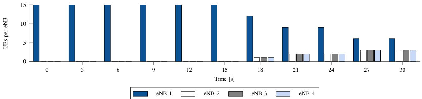
Fig. 19. Number of UEs connected to each eNB for a 30s test while they are distributed across the network to balance the traffic load.
