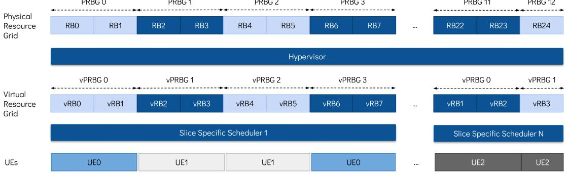
Fig. 7. Example of the different scheduling levels used by the 5G-EmPOWER Hypervisor.
