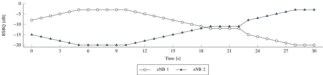
Fig. 18. Reported RSRQ by a UE with regard to 2 eNBs. When the current measured signal is lower than the one from another eNB a handover is performed.
