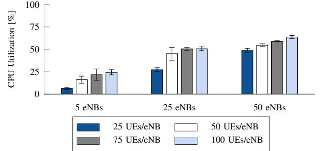
Fig. 10. CPU utilization of the *5G-EmPOWER* Operating System for an increasing number of eNBs and UEs.
