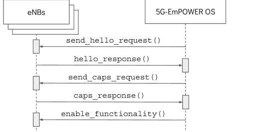
Fig. 4. Initial handshake between eNB and 5G-EmPOWER Operating System.
