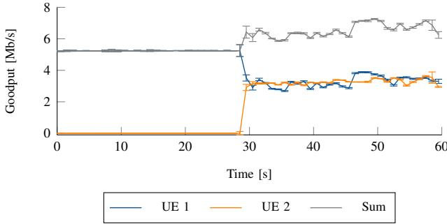
Fig. 16. Dynamic resource reallocation of 2 slices when a new UE is attached.
