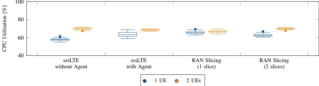
Fig. 9. Results in terms of CPU utilization of a vanilla eNB when introducing the *5G-EmPOWER* Agent in various setup configurations.
