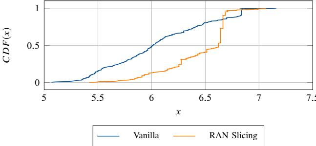
Fig. 11. CDF of the performance of one UE using the Vanilla and the RAN slicing system.
