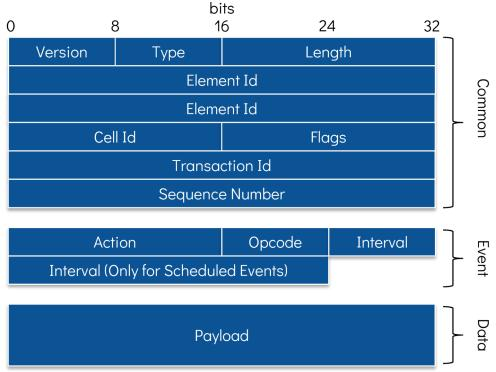
Fig. 2. The *OpenEmpower* message structure.
