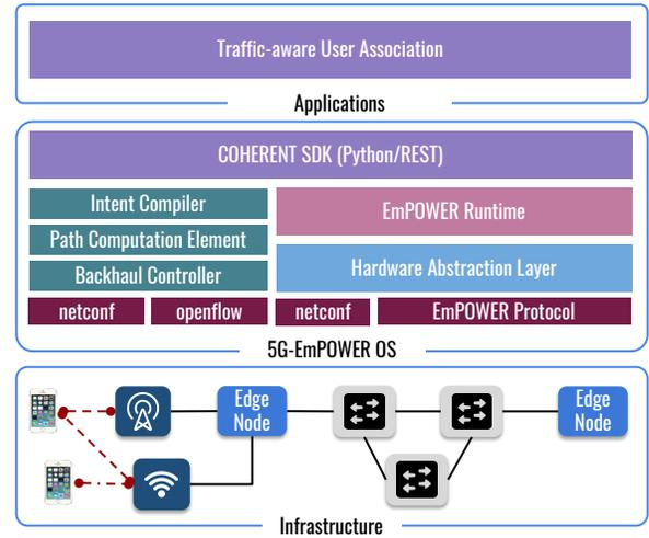
Fig. 5: The 5G-EmPOWER MEC-OS System Architecture.
