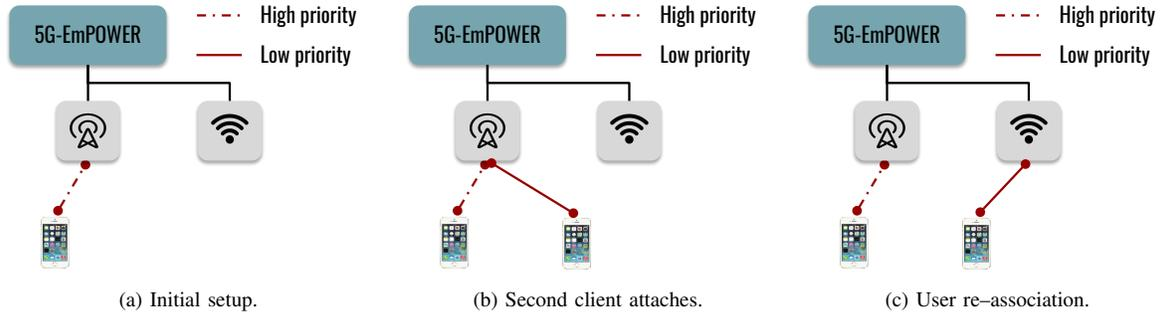
Fig. 6: Testbed setup. Initially only one client is active with a single high-priority flow served by the LTE eNB. When the second client attaches to the same eNB and starts generating a low-priority flow, the controllers detects a handover opportunity and associates the low-priority user to WiFi AP.
