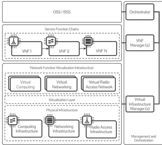
Fig. 6: Reference network function virtualization architecture [5].
