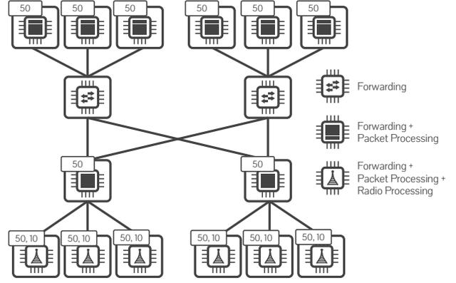
Fig. 1: Substrate network model used in our NFV architecture. The figure shows the three basic virtual resources: forwarding, packet processing, and radio access.
