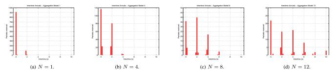
Fig. 6: Histogram of the AMEX messages' inter-arrival times for different values of the aggregation threshold N.
