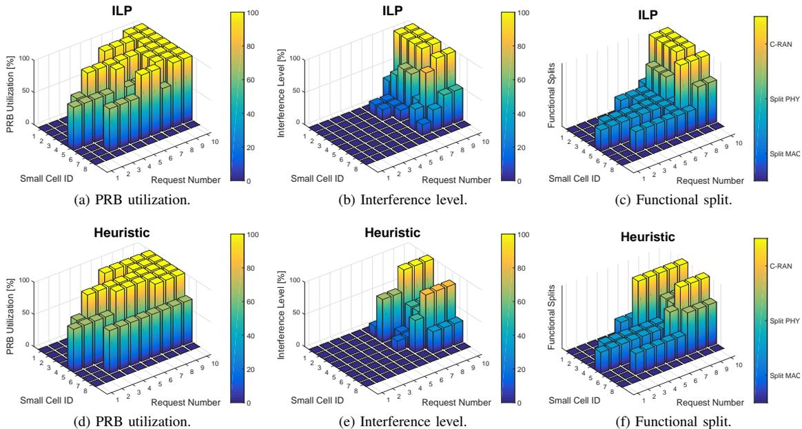
Fig. 5: PRB utilization, interference level and functional splits of the ILP-based and the heuristic algorithms.
