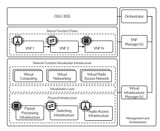
Fig. 6: Reference network function virtualization architecture [5].
