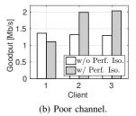
Fig. 9: Isolation across clients in different networks. Client 1 and 2 are in Tenant 1's network, while Client 3 is in Tenant 2's network.
