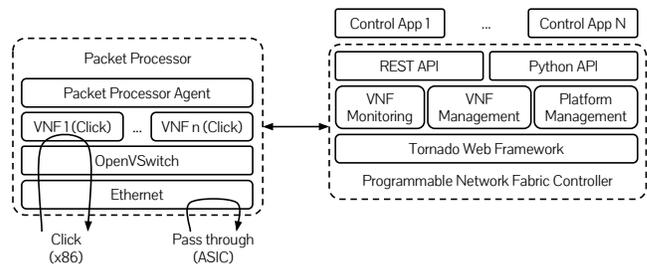
Figure 1: *Programmable Network Fabric Controller*.
