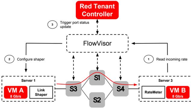
Fig. 3: The design of our performance isolation scheme relies on a distributed bandwidth shaping system combined with a reactive link labeling scheme and a label distribution mechanism exploiting existing OpenFlow messages (the *port status* message) although with minor modifications.
