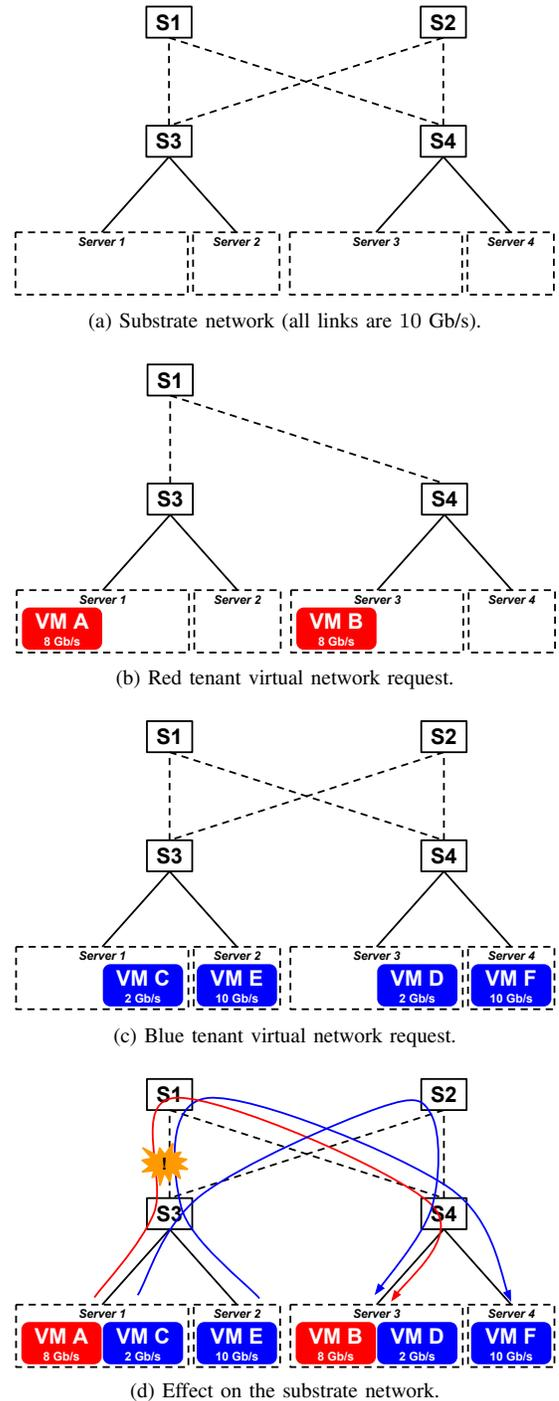
Fig. 1: Albeit full bisection bandwidth is available in the substrate network, the partial network view exploited by the two tenants in order to make routing decision can lead to sub-optimal use of the available resources.
