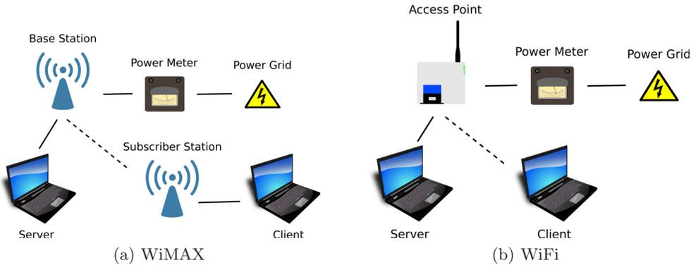
Figure 1: Network scenario used for the measurement campaign.
