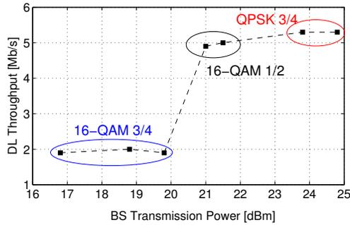
Figure 7: Goodput between BS and SS using different transmission power levels. The results refer to a saturated TCP connection.
