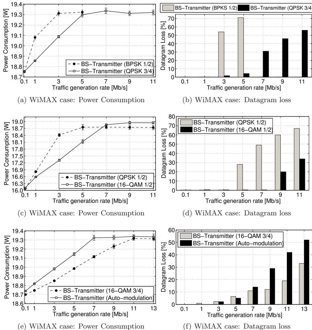
Figure 8: Average of power consumption at the BS (Transmitter) and datagram loss as a function of different traffic generation rate for different modulation types. Datagram size equal to 1280 bytes.
