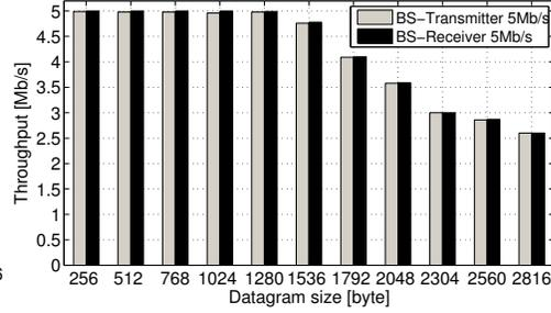
(b) WiMAX case: Throughput for the experiment with 5 Mb/s
