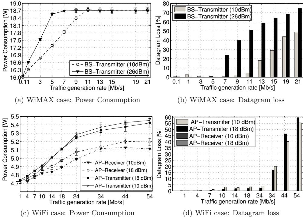
Figure 6: Average power consumption at the BS and AP and datagram loss as a function of different traffic generation rates for different transmission power levels. Datagram size equal to 1280 bytes.
