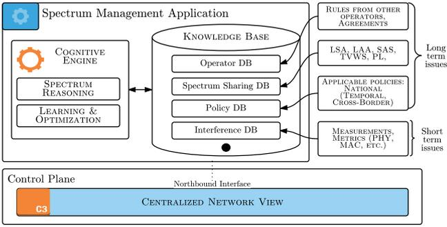
Fig. 3. Spectrum management application (SMA) detailed view
