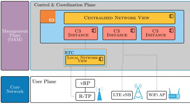
Fig. 1. COHERENT project wide architecture.
