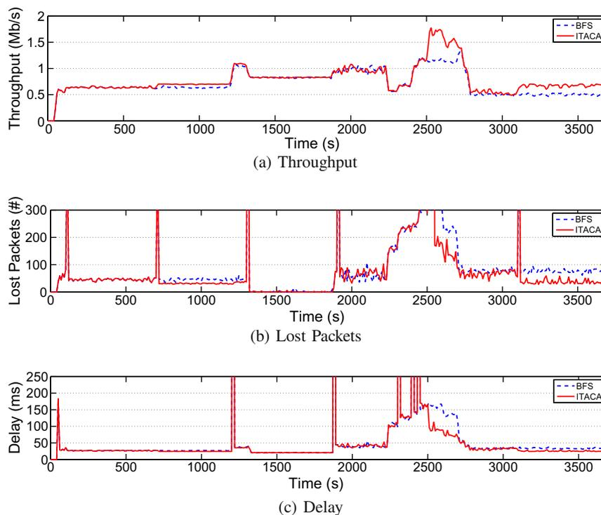
**Fig. 2.** Results of the simulation campaign involving 21 nodes distributed in a terrain of  $1000 \times 1000$  m. External interference has been taken into account by introducing 32 external nodes operating in the 5 GHz band.
