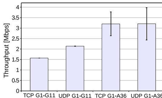
**Fig. 1.** Analysis of the cross-coupling effect between two co-located radios. The first and the second bar refer to the cases where both radios operate on the same band (2.4 GHz), while the third and the fourth bar refer to the case where the radios operate on two different bands (2.4 GHz and 5 GHz).
