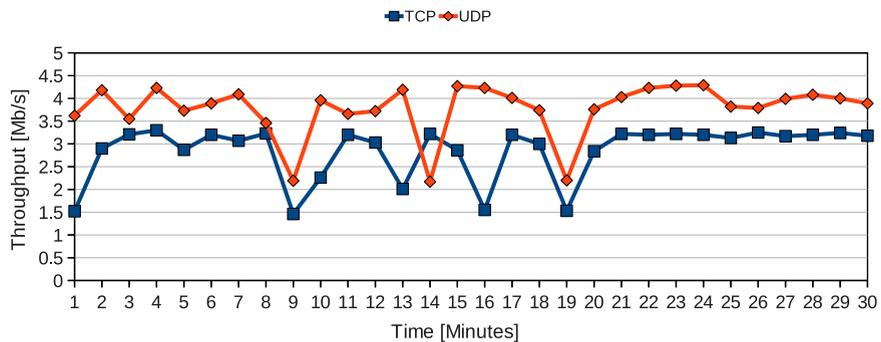
**Fig. 6.** Detail of the performance of the 3-hops path using both TCP and UDP traffic. The throughput oscillations around the 10th and 20th minute of the test are due to the channel scanning procedure implemented by ITACA.
