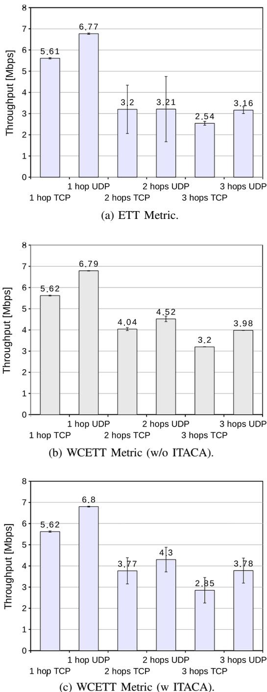
**Fig. 4.** Throughput degradation on a dual-radio testbed over string topology as the number of hops increases.
