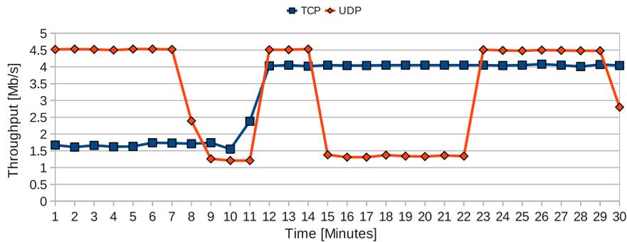
**Fig. 5.** Detail of the performance of the 2-hops path using both TCP and UDP traffic. The performance drops are due to fluctuations in the routing path caused by the inability of the ETT metric to choose channel diverse paths.
